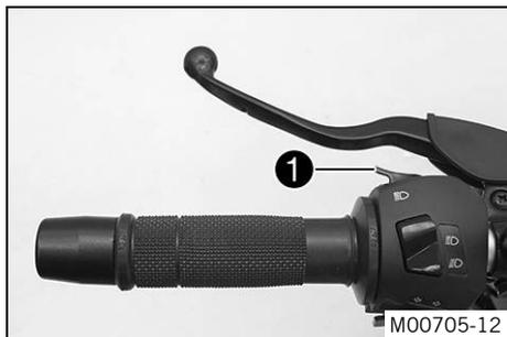
The high beam flasher button ❶ is fitted on the left side of the handlebar.
